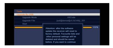
8. Software upgrade on process. **DURING THIS TIME**, please do not power-off the unit or perform any other operation that might disrupt the upgrade.
