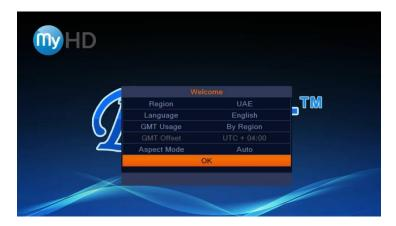
6. Once on the initial setup screen, Press EXIT and make sure that the front panel of the receiver will display NOCH message. This confirms that the receiver is into its factory settings state and software upgrade process can be performed
